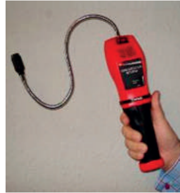
Figure 3 - Electronic leak detectors suitable for flammable refrigerants
